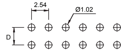
RECOMMENDED PCB LAYOUT
